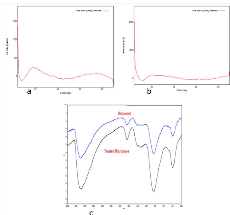
**Figure 4:** (a) XRD of Co-B-P catalyst in normal environment. (b) XRD of Co-B-P catalyst in microwave environment. (c) FTIR spectra of Co-B-P catalyst in normal and microwave environments.
