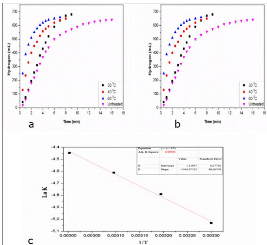
**Figure 2 (a):** Effect of different temperatures on hydrolysis of  $\text{NaBH}_4$ . **(b)** The nth order reaction kinetics of Co-B-P catalyst at different temperatures. **(c)** The first-order Arrhenius equation of Co-B-P catalyst.
