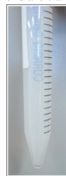
Figure 3: Image of stable translucent 0.5% aqueous dispersion of CNP in test-tube prepared by hydrolysis of cellulose with 40 wt. % SA at 80°C followed by sonication
