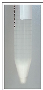
Figure 4: Image of white sediment of cellulose microparticles on bottom of test-tube precipitated from 0.5% aqueous dispersion containing mixture of CNP and MP prepared by hydrolysis of cellulose with 40 wt. % SA at 60°C followed by sonication.
