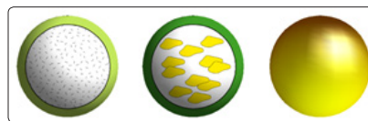
Figure 1: Schematic drawing of Microcapsules and Microspheres. From left to right: Microcapsule with solution as core, Microcapsule with cell suspension as core, Microsphere with matrix encapsulated active agent
