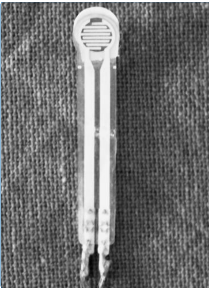
Figure 1: Flexiforce Resistive Sensor of diameter 0.16”
