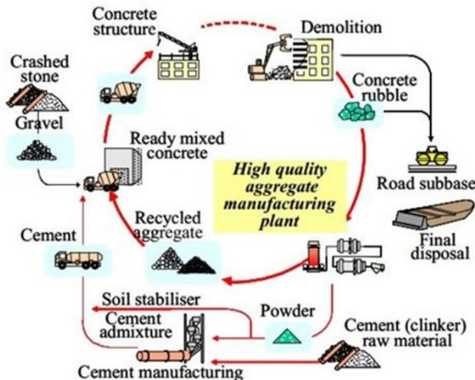
Figure 4: Process of waste concrete recycling
